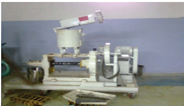
Figure 2 Compression machine for extracting oil from Jatropha seeds (color figure available online).
