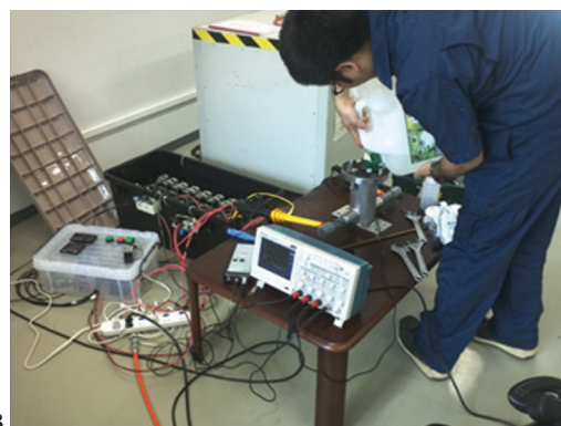
Fig. 1. Pressure chamber. View from above (A) – the chamber generating the pressure shockwaves (50 MPa to 60 MPa) by discharges of high voltage (3.5 kV). Setting the electrical equipment associated to the pressure chamber (B).
