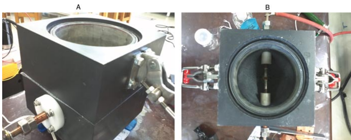
Fig. 1. Side view (A) and view from above (B) on lockable strengthened metallic vessel for high-voltage underwater discharges causing pressure 50–60 MPa shock waves, prototype number 4, with an inner spherical volume of 2 L, a minimal vessel thickness of 2 cm, and copper electrodes.
